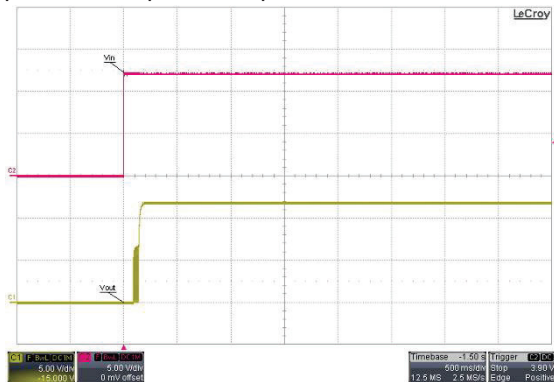
Typical Start-Up and Output Rise Characteristic
