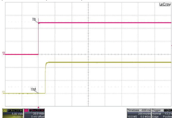
Typical Start-Up and Output Rise Characteristic
