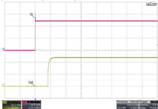
Typical Start-Up and Output Rise Characteristic
