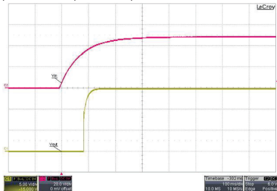
Typical Start-Up and Output Rise Characteristic
