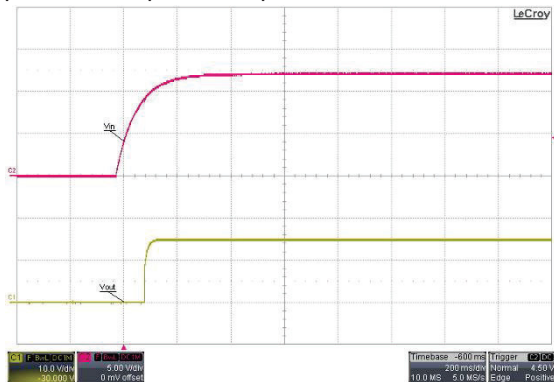
Typical Start-Up and Output Rise Characteristic
