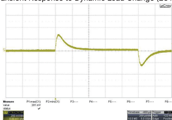
Transient Response to Dynamic Load Change (25%)
