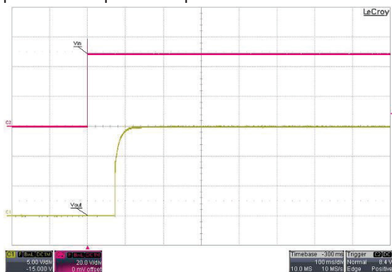
Typical Start-Up and Output Rise Characteristic
