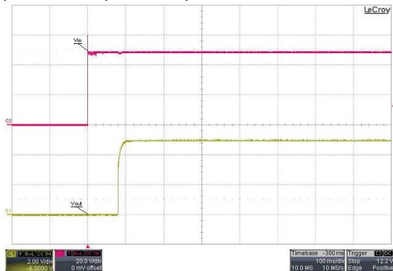
Typical Start-Up and Output Rise Characteristic
