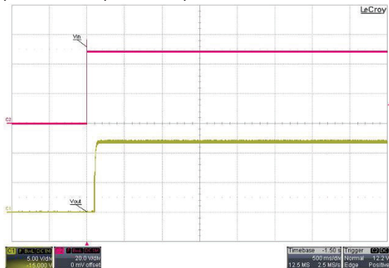
Typical Start-Up and Output Rise Characteristic
