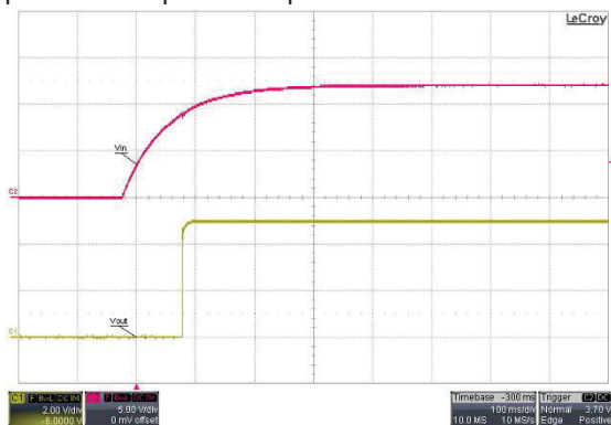
Typical Start-Up and Output Rise Characteristic
