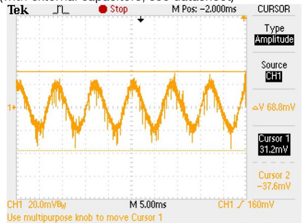
Typical Output Ripple and Noise at 230 Vin (with external capacitors; see datasheet)
