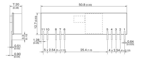
Dimensions in mm (inch) Tolerances x.x  $\pm 0.5$  (x.xx  $\pm 0.02$ ) Tolerances x.xx  $\pm 0.25$  (x.xxx  $\pm 0.01$ ) Pin dimension tolerance ±0.1 (±0.004)
